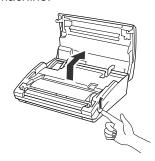
3. Press the roller's tabs outward and lift the roller out of the fax machine.
